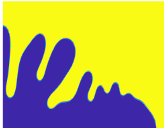
Figure 5: Simulation of nickel dendrite (isotropic) with nonlocal solidification model. The model is simulated on a coarse mesh and phase-field solution has sharp interfaces up to mesh resolution ( \sim 1-2 cells).
